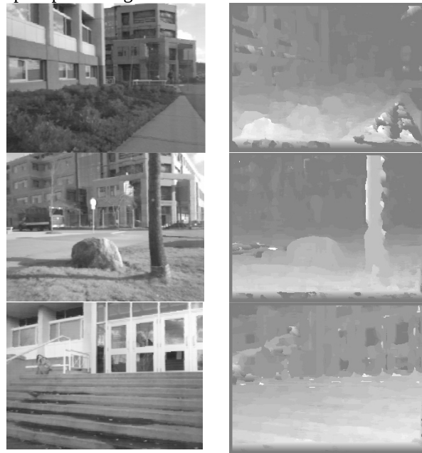
Fig. 6. Test stereo images and disparity maps from the proposed architecture
